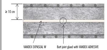
VANDEX EXPASEAL W waterstops must not be stretched during installation.
